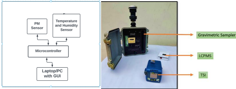
Figure 1. Schematic diagram of the sensor module and the pictures of the instruments used in this study
